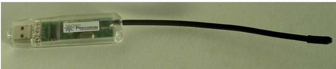
*The wireless USB-Dongle (here Version for 433 MHz (Europe/Asia/Africa) with built-in Antenna).*
