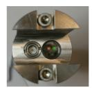
Picture: IR converter and logger top (without connected antenna)
