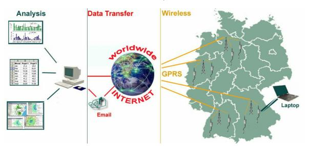
Picture: Structure of GPRS data transmission
